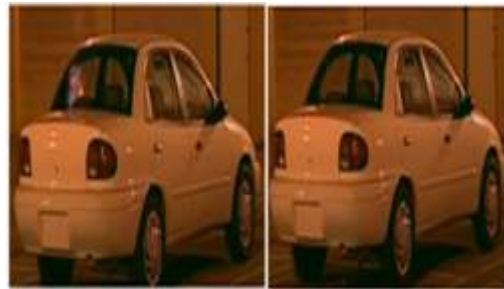
Figure-3: Picture showing no damage after hydrogen fire was over in 100 seconds ( https://www.youtube.com/watch?v=OA8dNFivAFQ ).
