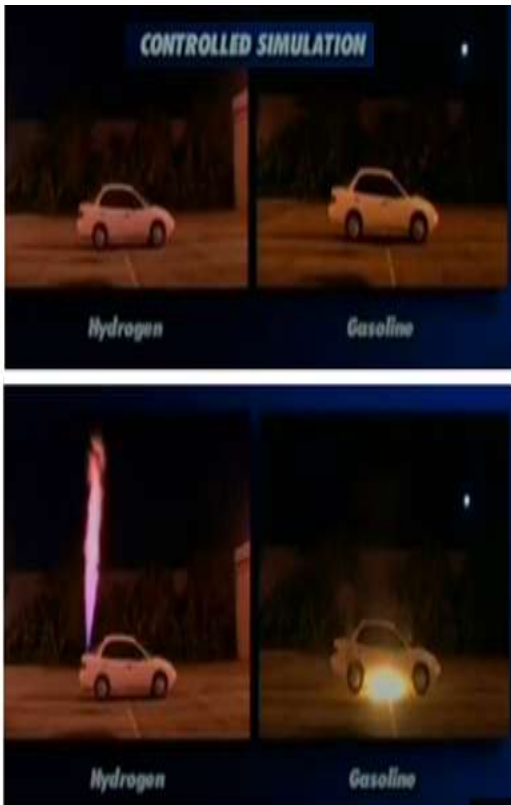
Figure-1: A picture from a video of the two car fires from the leak at one minute after ignition ( https://www.youtube.com/watch?v=OA8dNFivAFQ ).
